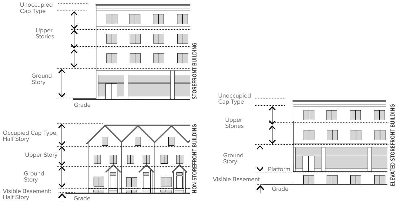
Figure 660(57) Measuring Building Height
